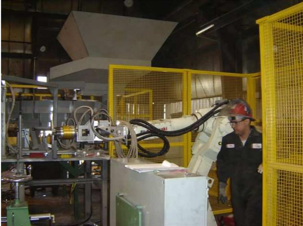
The end-of-arm tooling was designed so that both the ID robot and the OD robot tooling was the same with the exception of the grippers.
