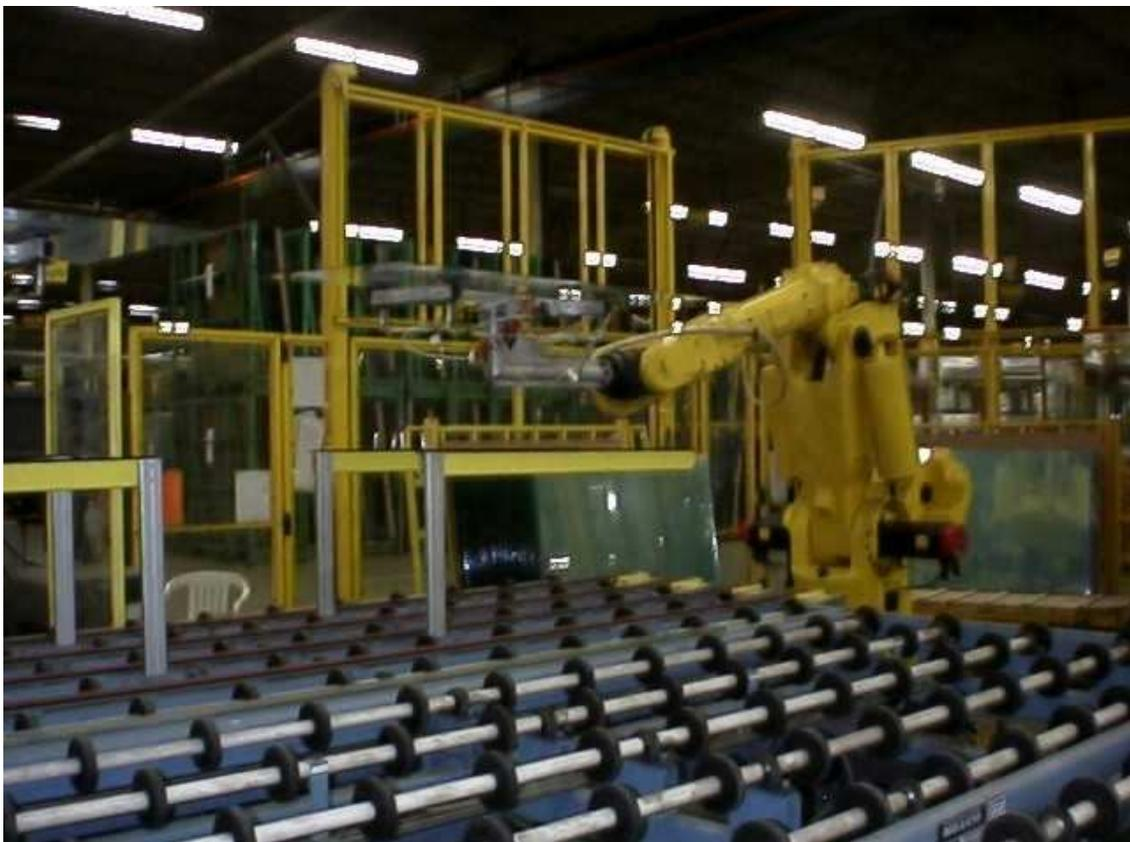
There are two robots at the exit end of the line named Unload Robot A and Unload Robot B. These robots pick processed glass from the line and stack it on pallets. The following picture shows one of the unload robots.
