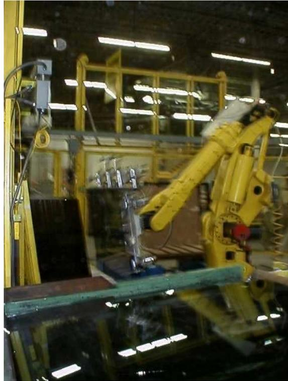
The two mask robots are located in the center of the coating line. One of these robots is the mask load robot. It picks up a mask and places it on the line. When the mask is no longer needed, the mask unload robot picks the masks off of the line and places them on a pallet. The following picture shows one of the mask robots.
